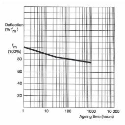
Graphs N° 2 Evolution of P<sub>45</sub> after ageing at 150°C totally compressed (measured at room temperature).
